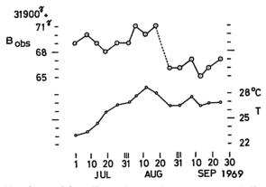
Fig. 2. Weekly observed base-line values and temperatures of Kanoya's No. 1 Z-variometer in July, August and September of 1969.
