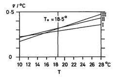
Fig. 3. Temperature coefficients of Kanoya's No. 1 Z-variometer.
