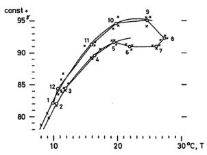
Fig. 6. Temperature-dependence of base-line values of Kanoya's No. 2 Z-variometer with the drift, 1.133 t + Dc, subtracted.
