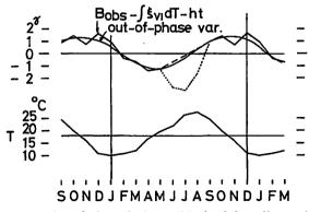
Fig. 10. Mean annual variation of the residual of base-line values shown at the top of Fig. 9 (upper) and temperatures (lower). A smooth curve in the upper part is the out-of-phase variation with respect to the annual term of temperature change when  $k=0.0819\gamma/month/^{\circ}C$ .
