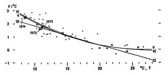
Fig. 8. Temperature-dependence of temperature coefficient of Kanoya's No. 2 Z-variometer. For III, V and VI, see Eqs. (9), (12) and (13).
