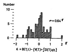
Fig. 6. Distribution of the difference between observed values B(T, t)and calculated ones  $V(T) + \int D(T) dt$  of the base-line value at Kanoya for the year 1966.
