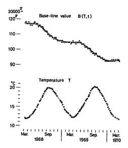
Fig. 8. Observed base-line value B(T, t) (corrected by the magnitude of gap) and room temperature T at Kakioka.
