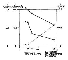
Fig. 11. Relation between each coefficient and a practical measure of temperature dependence,  $\overline{|dV(T)/dT|}$ .
