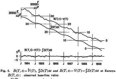
V(T): temperature dependence  $\int D(T) dt$ : drift
