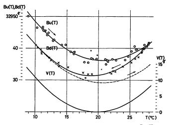
Fig. 3. Apparent temperature dependence of base-line value  $B_u(T)$  for the months of ascending temperature and  $B_d(T)$  for those of descending temperature and their mean V(T) at Kanoya. Broken curve expresses  $B_u(T)$  of the next year's which succeeds the  $B_d(T)$ , the former being not corrected for the year-to-year change.
