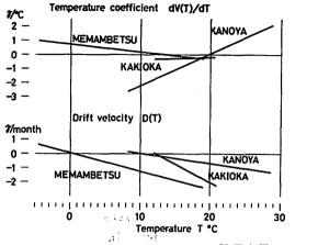
Fig. 10. Summary of temperature coefficients dV(T)/dT and drift velocities D(T) at three observatories.
