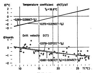
Fig. 4. Temperature coefficient dV(T)/dT and drift velocity D(T) at Kanoya. Broken lines are those obtained in Section 3.
