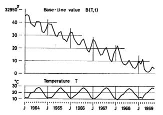
Fig. 1. Monthly means of observed base-line value B(T, t) and room temperature T at Kanoya.
