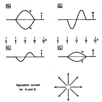
Fig. 5. Schematic diagram showing fundamental type of diurnal variation,  $H_0$  and  $D_0$  and additional field,  $H_1$  and  $D_1$ . The lower figure is the equivalent current system for  $H_1$  and  $D_1$ .
