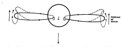
Fig. 20. Schematic picture describing the excitation of transverse hydromagnetic waves on the morning and evening sides of the carth. (after Wilson and Sugiura)
