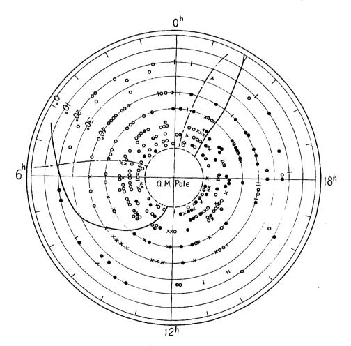
Fig. 2. Occurrence distribution of ssc's with clockwise (black circles), counterclockwise (open circles), linear (bars) and irregular (crosses or half open circles) rotations of the horizontal disturbance vector.
