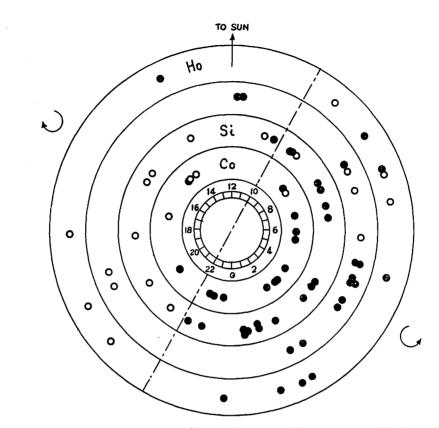
Fig. 3. Occurrence distribution of ssc's with counterclockwise rotation (black circles) and with clockwise rotation (open circles) of the magnetic vector for stations in the northern hemisphere. The regions of opposite directions of rotation are separated by the meridian plane through 10 and 22 hours in local time. (after Wilson and Sugiura)
